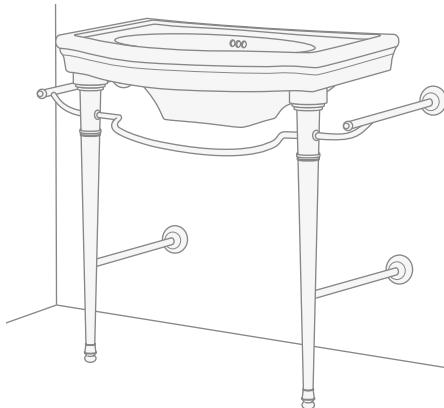
**13)** Seal the area between the basin and the wall with silicon.
