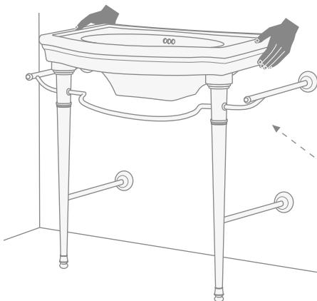
**10)** Keeping the basin in the correct position with the aid of the level, mark the position of the holes for fastening the basin support S-shaped brackets.
