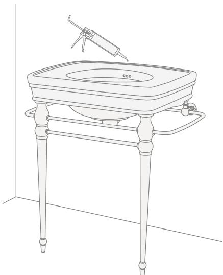
**15)** Position the basin once again, inserting the back part between the brackets and the wall.
