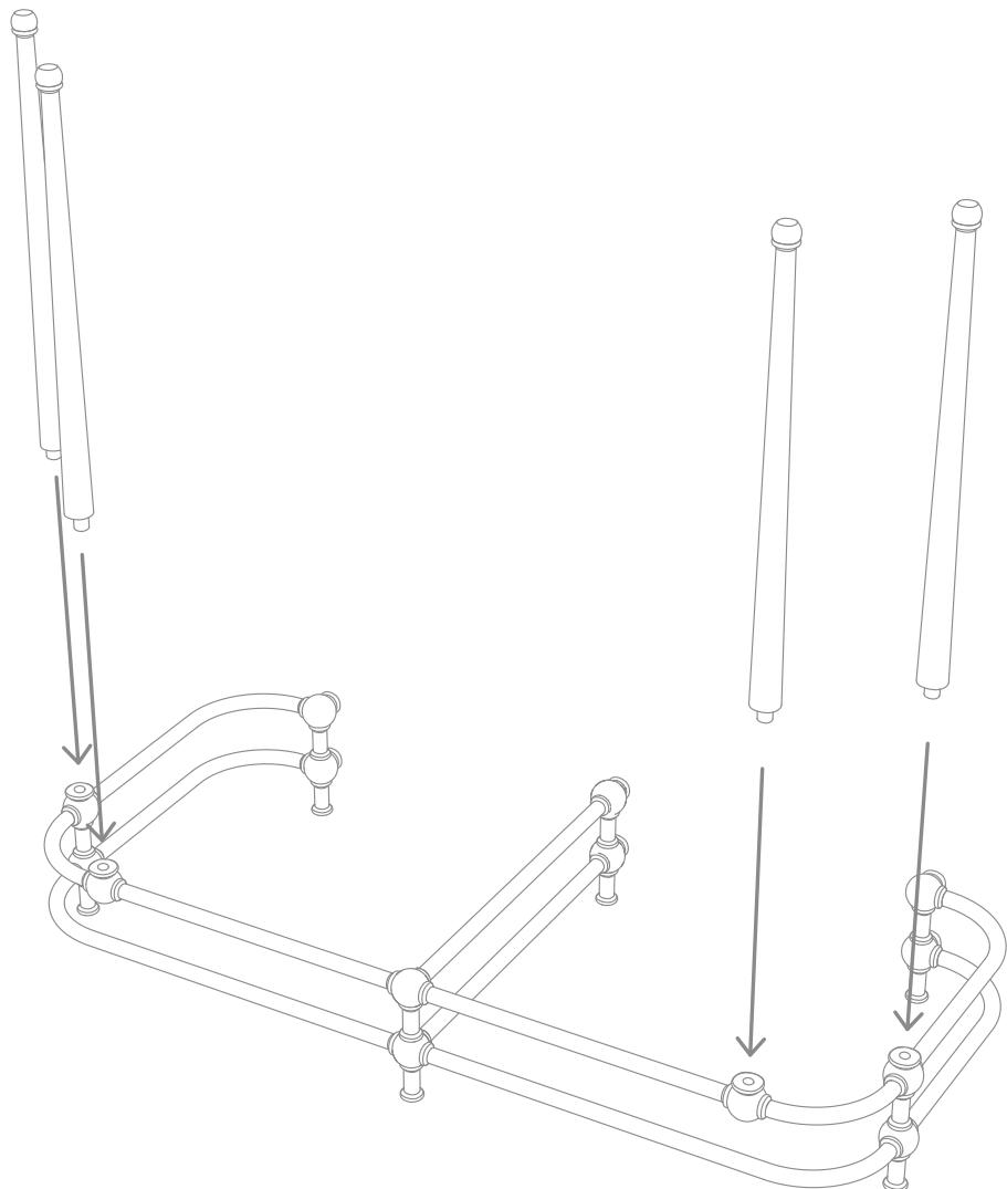
**4)** Now you can turn the console upside down, with its four legs just mounted and place it against the wall. Use the cardboard template (L: supplied) to mark the fixing points of the console.
