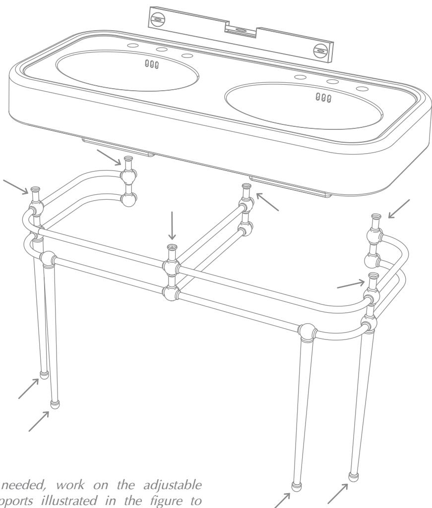
**10)** Mark the four holes where the washbasin will be fixed to the wall. Remove the washbasin and drill the four holes according to the above marks.
