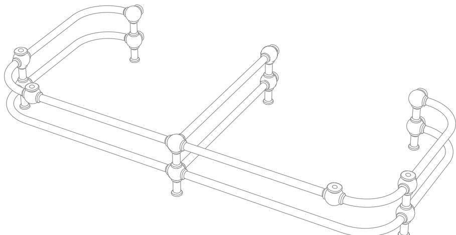
**3)** Screw the four legs of the console (B) into the points indicated on the frame.
