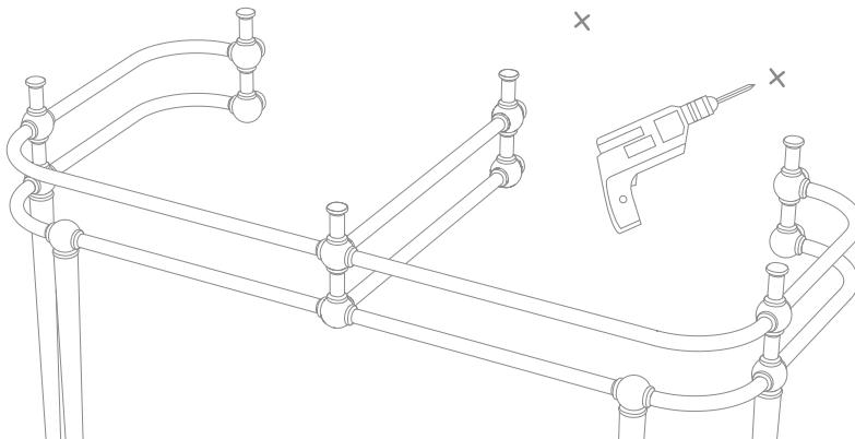
**11)** Insert the wall dowels into the holes, reposition the washbasin and fix it with the screws and the plastic washers (H+I) that are also supplied.
