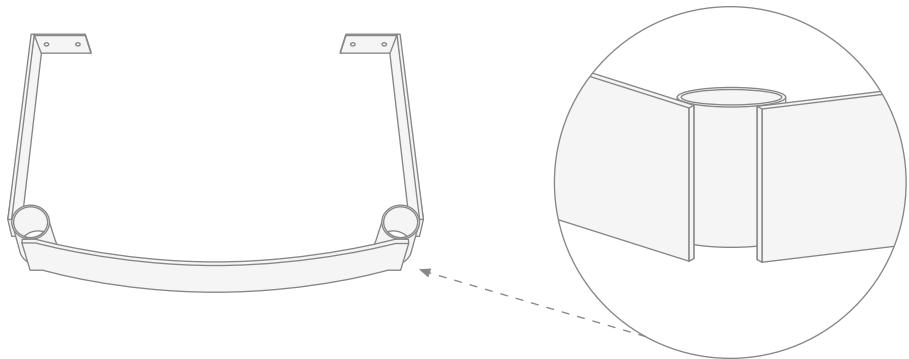
**2)** Insert the leg with its threaded bar in the structure so that the leg reaches its contact position from the lower part of the structure.
