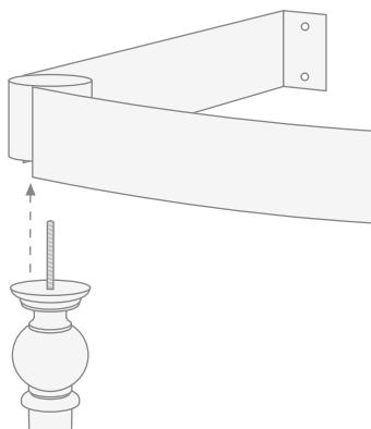
**3)** Screw the support on the threaded bar from the opposite part of the structure until the leg is locked. Repeat these operations for both legs.
