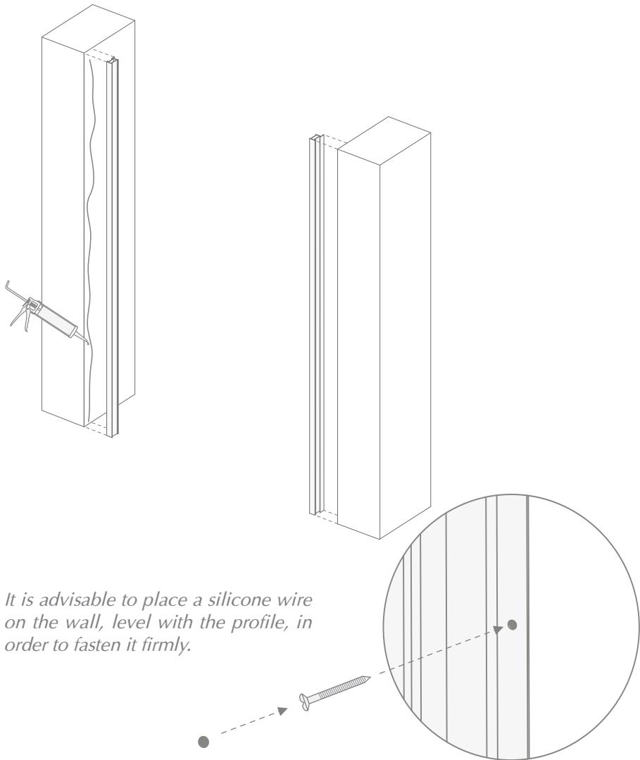
**7)** Centre the shower door (holding the sliding part closed) and slide the frame of the door on the profiles installed and secure everything with the self-threading screws (provided) from the inside.
