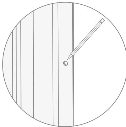
**4)** Remove the profile compensators and drill where the four points are marked out.
