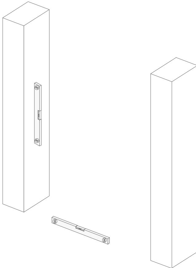
**2)** Position the predrilled wall profiles (B) and use a spirit level to check that these are perfectly plumb and at right-angles to the wall.
