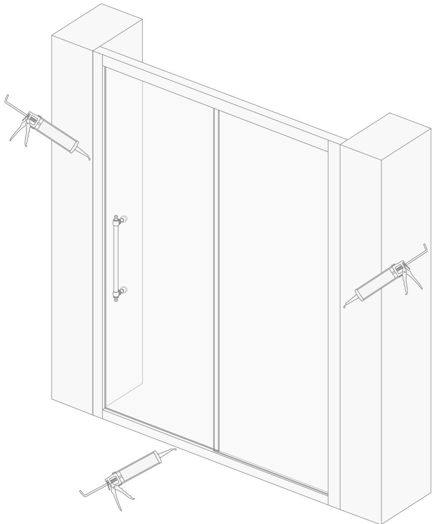
**15)** Using a piece of paper and alcohol, carefully clean off all the excess silicone around the shower enclosure.
