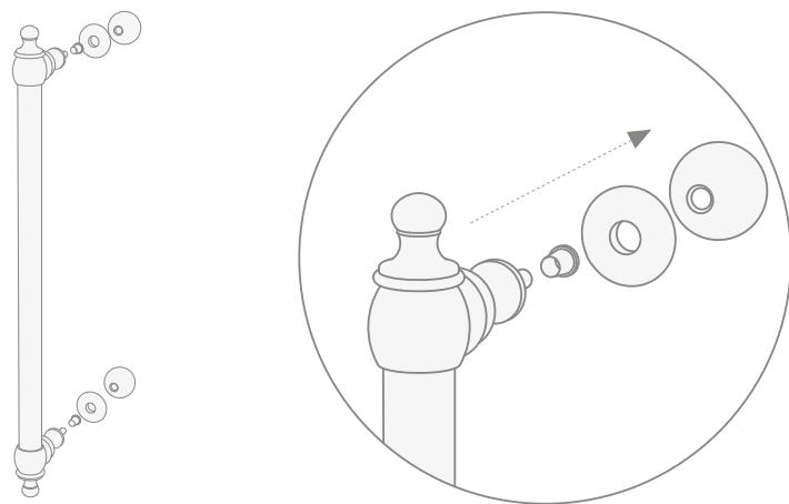
**11)** Insert the handle (H) into the holes on the glass pane of the shower enclosure (sliding).
