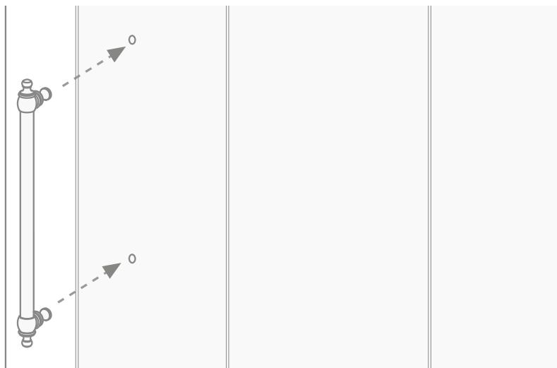
12) You can now fix the handle, from the inside, by screwing the parts unscrewed before from both parts back in.
