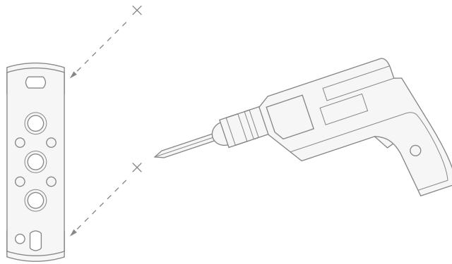
**4)** Insert the rawl plugs, position the plate and fasten it to the wall taking care to pass the power supply cables through the hole provided.
