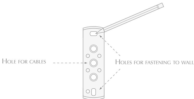
**3)** Remove the plate and drill the holes in the wall as just marked.
