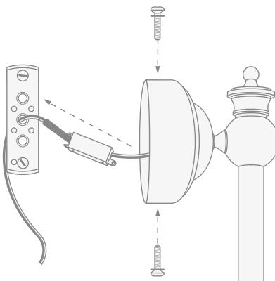
**8)** Pay attention to the fact that near the fastening hole in the bottom part of the lamp body there are two holes: one is for fastening and the other is the hole provided to obtain protection class IP21 together with the special optional kit.
