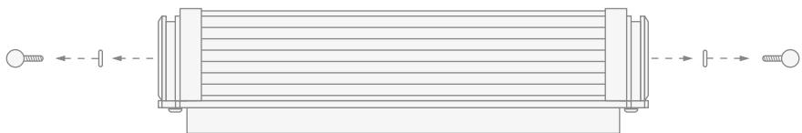
Remove the lamp glass slackening the two knobs (and corresponding washers) at the ends of the lamp.
