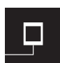
Pre-wired with approx 150mm of cable from the head. Connection to be done inside the pole
